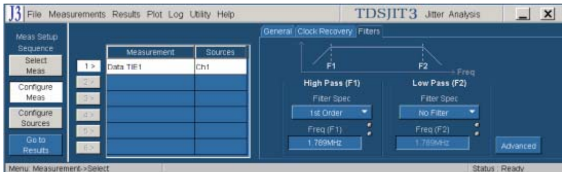
Figure 98: Configuring filters for a 1.5 Gbps SAS device
