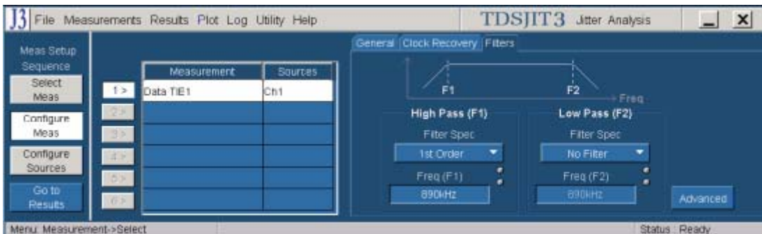
Figure 97: Configuring filters for a 1.5 Gbps SAS device
